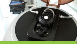
On-line measurement option Kinetic of aggregation Portable instrument (<12 kg)
