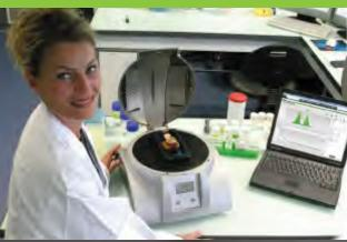
Based on a patented innovative technology developed in collaboration with the French Institute of Petroleum (IFP), the VASCO particle size analyzer is a unique instrument for nano to micro particle size measurements in suspensions. The measurement principle is based on Dynamic Light Scattering (DLS) of back-scattered light.
